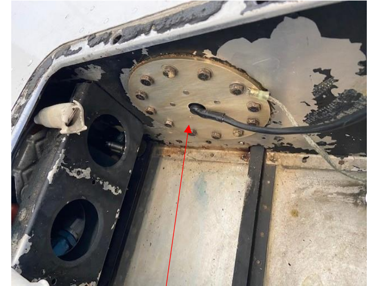
CiES Fuel sender and bracket installed
